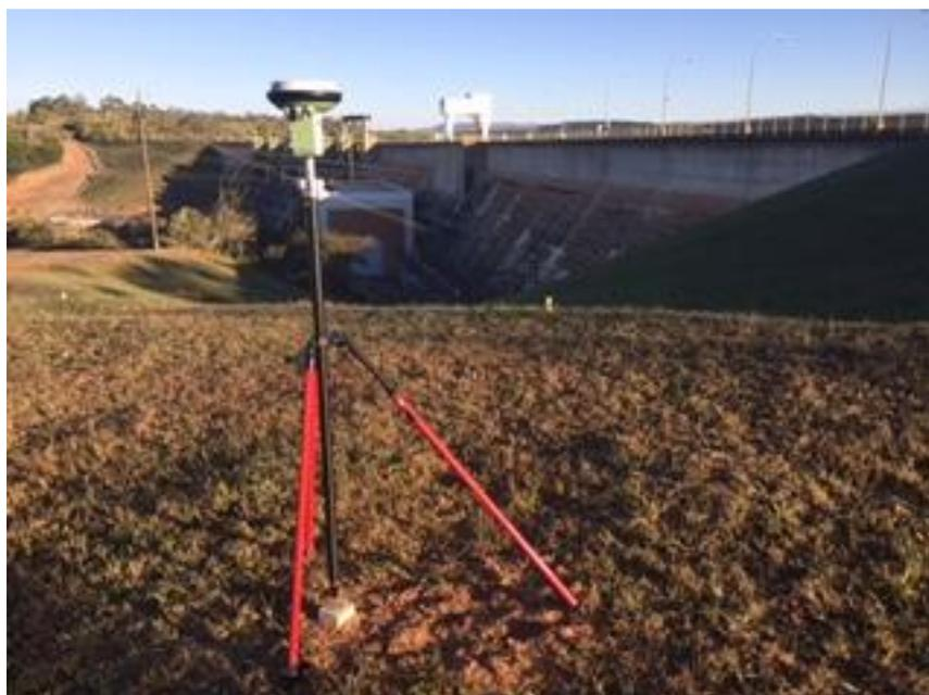
Figura 21: Receptor GNSS rastreando marco M3.
