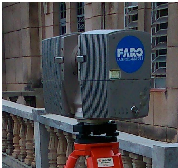
Figura 12 – Laser Scanner Terrestre Faro Photon 80
